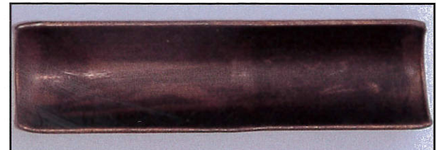
Oil Fouling Prior to Treatment
